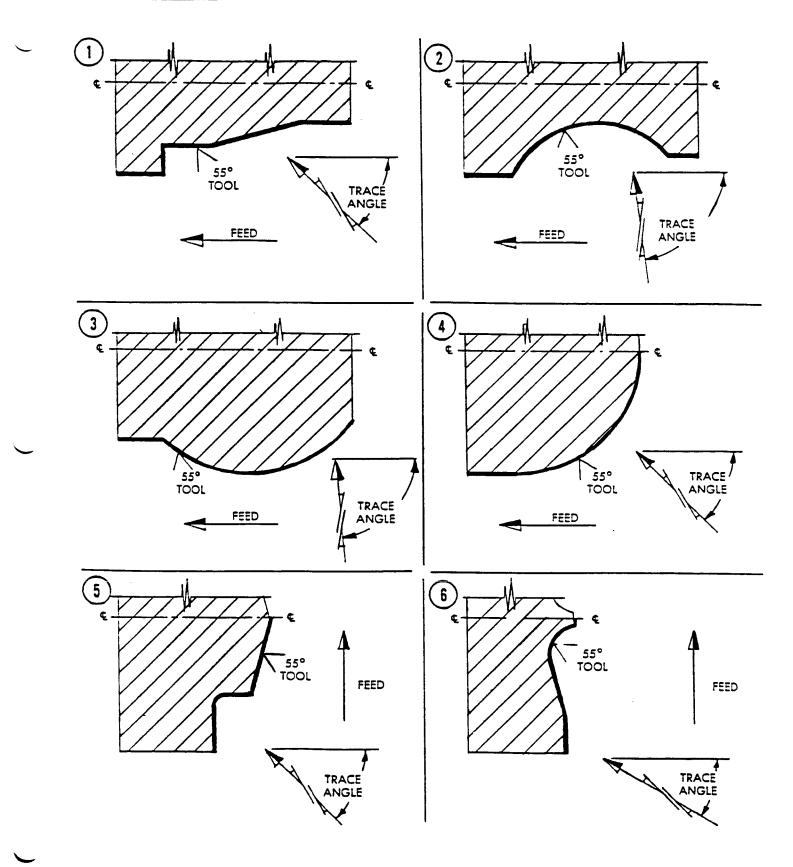
GENERALLY, THE TRACE ANGLE SHOULD BISECT THE SMALLEST CONTAINED ANGLE IN THE TRACE PATH.
