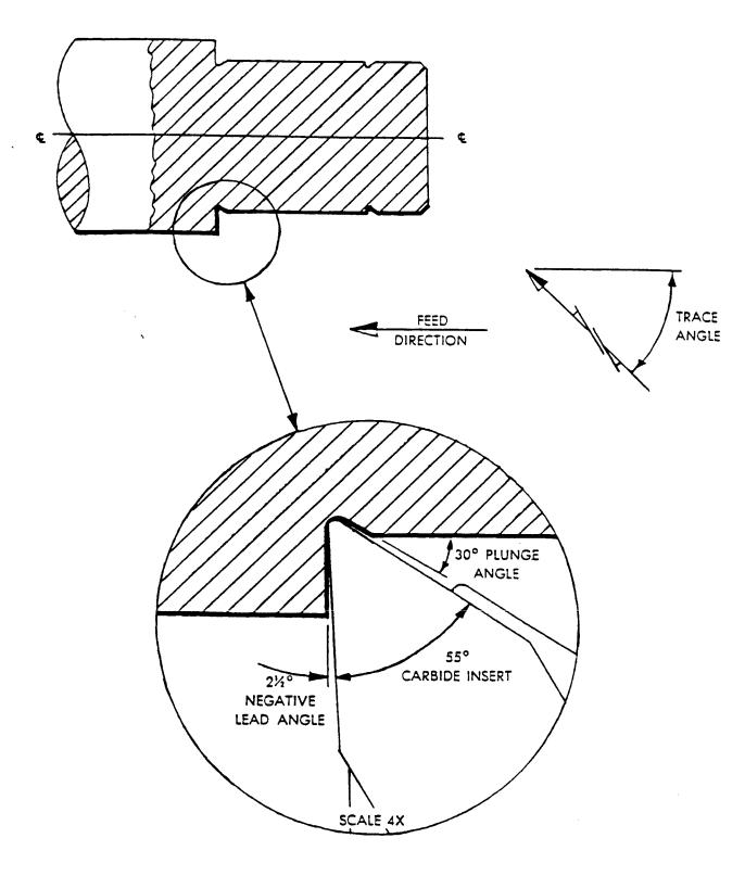
SUGGESTED METHOD FOR TRACING UNDERCUTS IN SHAFTS
