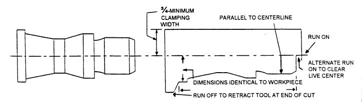
Sawing and filing to layout lines is often acceptable, although milling, grinding or polishing may be needed in some cases. The contoured edge should be square to the surface, and must be free of nicks and burrs. Remember that an error in template dimensions can be doubled when tracing a diameter!
